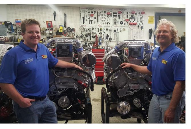
the engine so it can be used in saltwater. The engine has twin 4.0-liter Whipple superchargers with an engine management system from A.E.M. that has proprietary firmware and it makes 1,850 hp on 91-octane gasoline. Goodwin Competition also designs the engines with maintenance in mind. Regularly serviced accessories are easy to get to. "You don't have to take apart 10 things to get to one thing behind them," Goodwin said.
